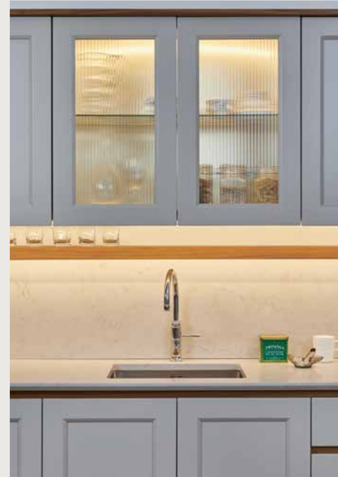
Walnut Arcadia Shelves conceal continuous LED strips, which bounce light off the wall cladding to illuminate the countertop.
